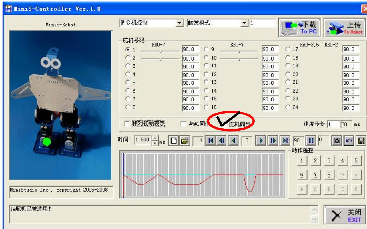
Synch can make servo work simultaneously corresponding to software Slider, spin box or Edit box setting.
