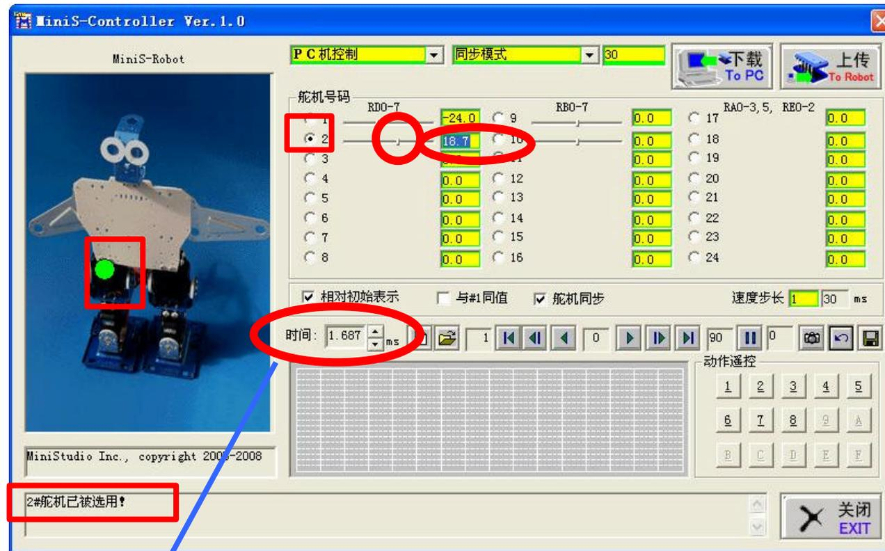
Click the picture you may find Servo position and use software Slider, spin box or Edit box setting to adjust servo angle.
